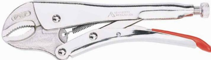
All pliers body of sheet steel, adjustable clamping range, toggle lever clamping and quick action lever release, surface nickel plated.
